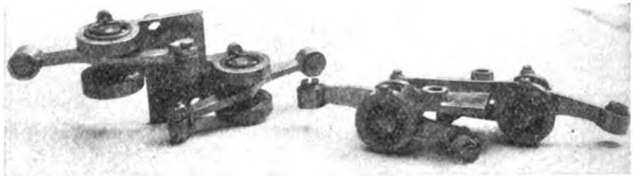
BALL-BEARING BRONZE ROCKER ARMS WHICH ACTUATE THE VALVES.
